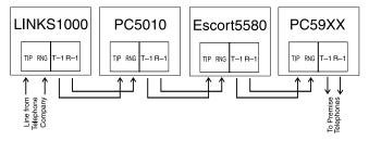
For example, if you are installing a PC5008 with a LINKS1000 and a PC5928 Intercom module, connect the incoming line to the LINKS1000, then from the LINKS1000 to the PC5008, then from the PC5008 to the PC5928 Intercom and then from the PC5928 to the house telephones.
